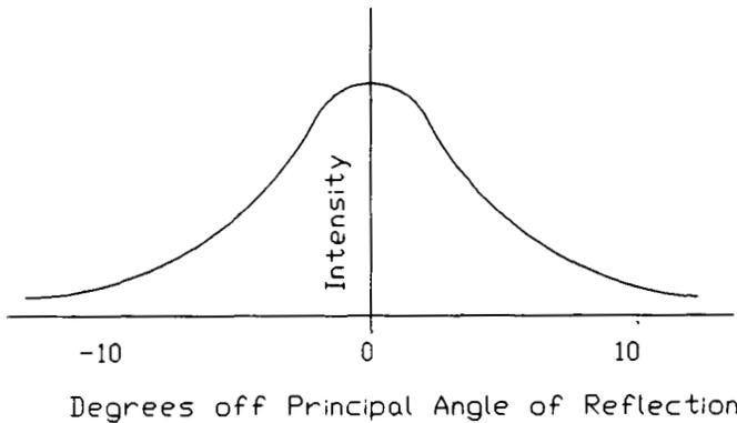
parameters. A specularly reflected (or refracted) ray is distributed in a cone with an angle theta and according to a cosine to the power n law. These four numbers are theta, n for reflection and theta, n for refraction respectively. If you want to add your own attributes, we recommend making these numbers "60 4.0 60 4.0."
